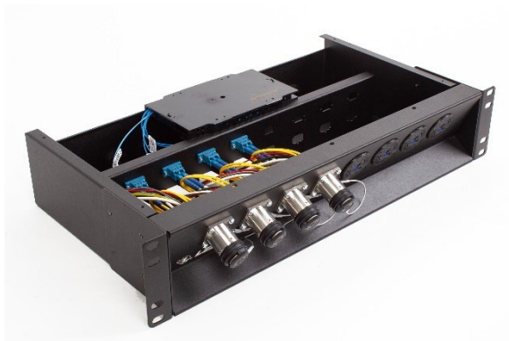
Internal arrangement of WST.ST.X0D4-DLCF-S-C1-4M
